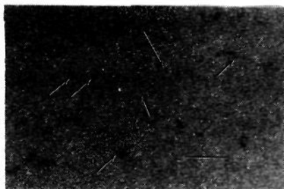
Figure 1. Bright-field TEM of "dimeric" HPT 4d . The spacing between the dots is about 2–3 nm (different orientations of the dimers) and is consistent with the separation indicated from an inspection of molecular models of an extended conformation of 4d . The bar represents 20 nm.
